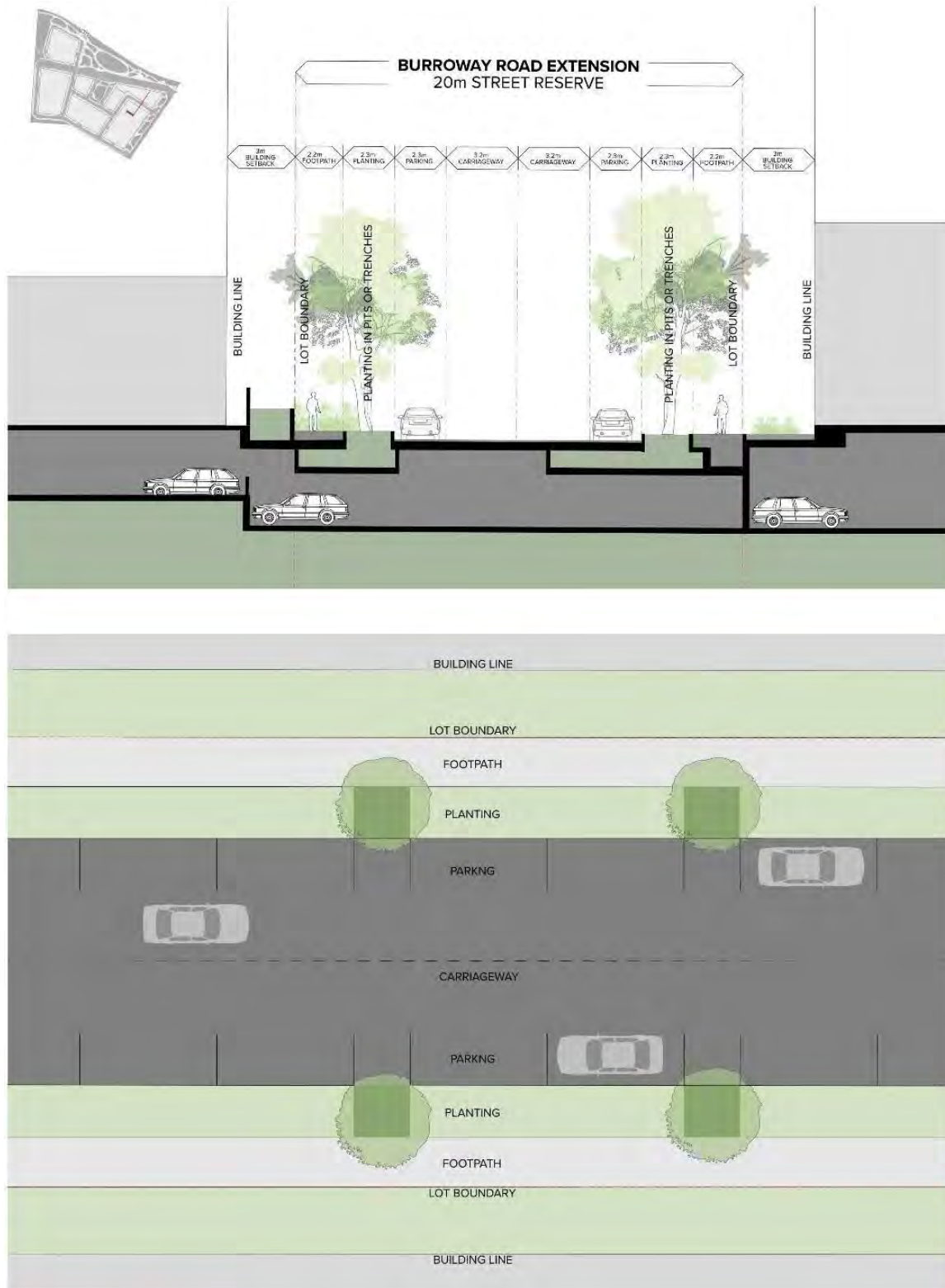
Figure 4 – Burroway Road (western extension) Indicative Cross-section
