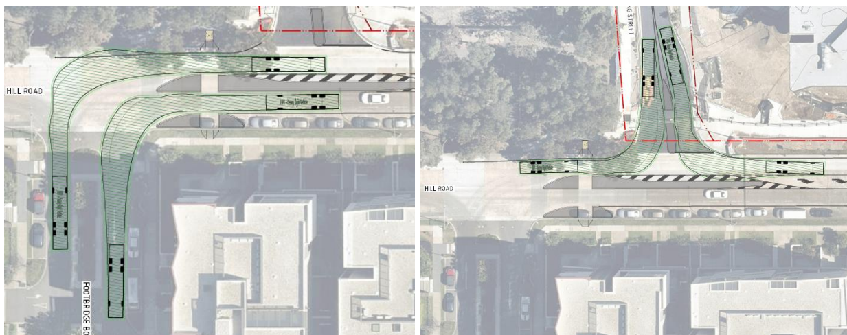
Figure 7: Swept path diagrams of a 12.5m Heavy Rigid Vehicle at the proposed median island in Hill Road north of Footbridge Boulevard
