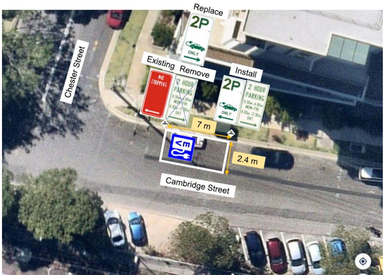
Figure 3: Sign and pavement marking plan for the proposed EV space at 28 Cambridge Street, Epping
