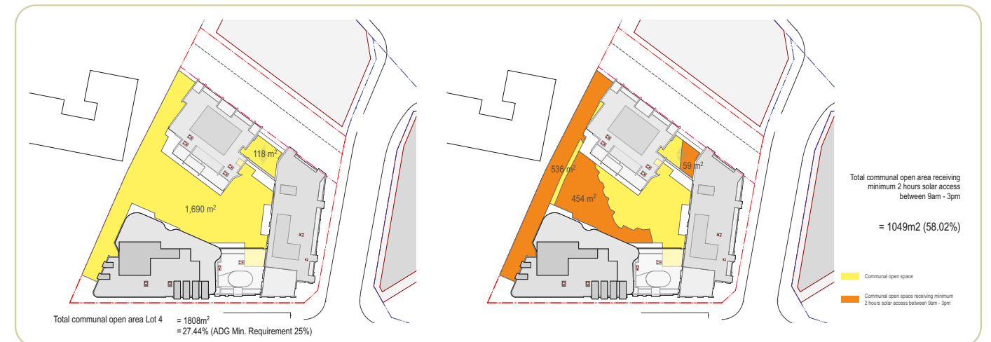
Figure 17. Lot 4: Solar access to communal open space 21 June 9am – 3pm (Source: Turner)
