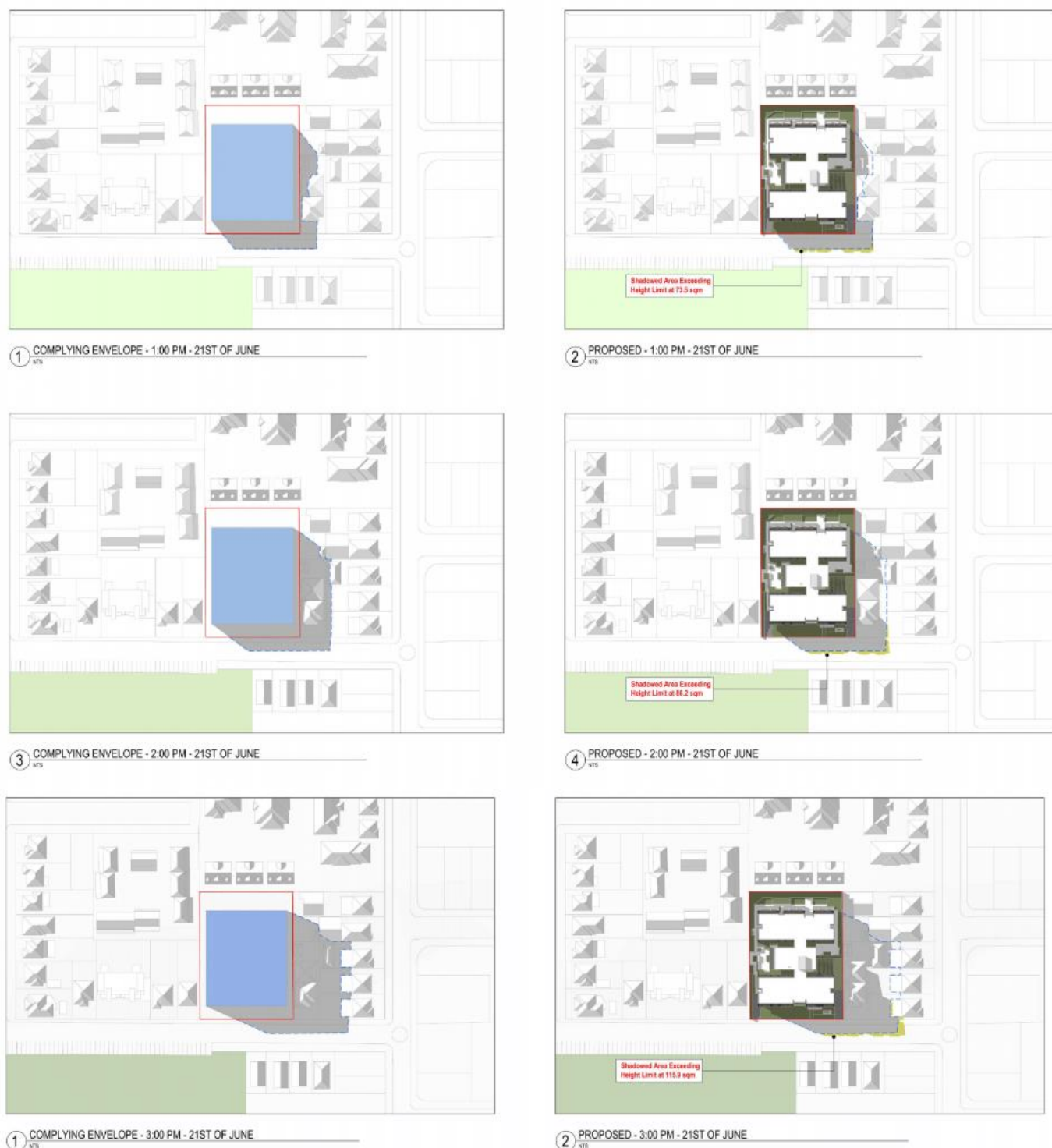
Figure 19 Overshadowing Analysis during the winter solstice
