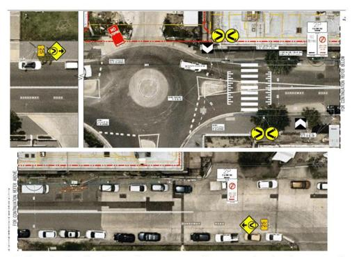
Figure 3: Plan showing the signs and pavement markings associated to the proposed raised pedestrian crossing in Burroway Road, Wentworth Point
