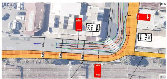
Figure 5: Swept Path plan of a 12.5m long rigid bus travelling through the bend between Station Street East and Marion Street, Harris Park
