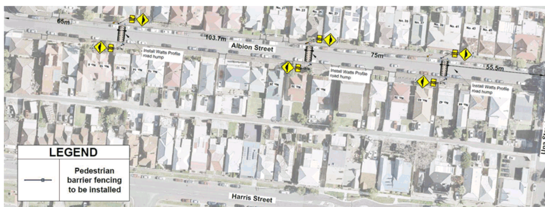
Figure 2: Concept plan of the proposed speed humps in Albion Street, Harris Park
