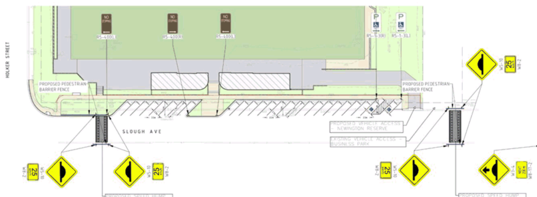
Figure 2: Design plan for the proposed speed humps and angle parking spaces in Slough Avenue, Silverwater
