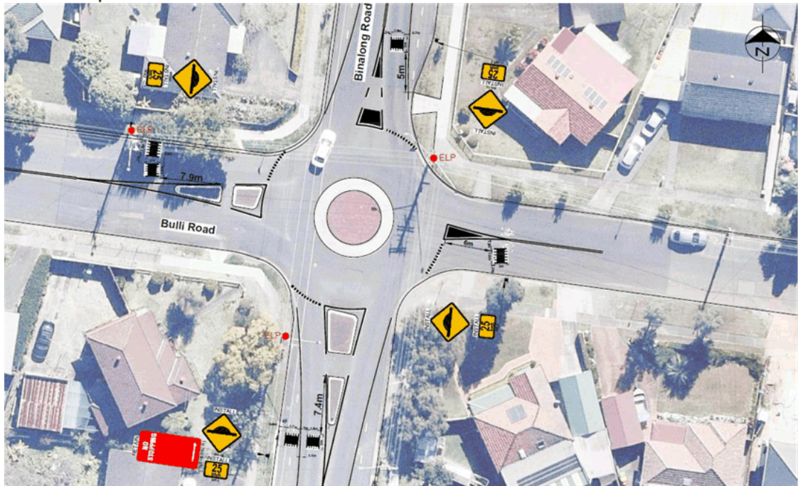
Figure 2: Concept plan of the proposed speed cushions at the intersection of Bulli Road and Binalong Road, Toongabbie
