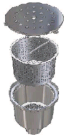
Floor Drain Basket Armator Install to floor as per hydraulic engineers details and ensure epoxy floor paint is applied prior to fitting off drain to ensure complete waterproofing of the existing floor slab
