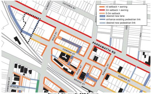
Figure 5: Site specific DCP Controls
