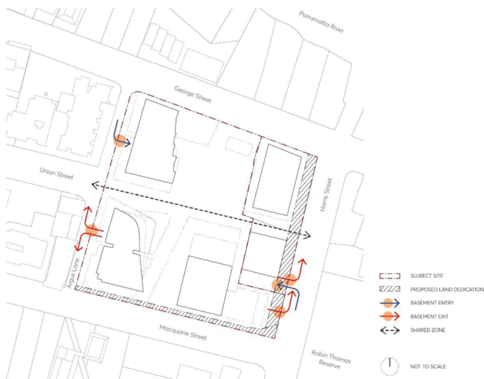
Figure 4.3.3.7.30 – Control diagram: Vehicular Access and Servicing
