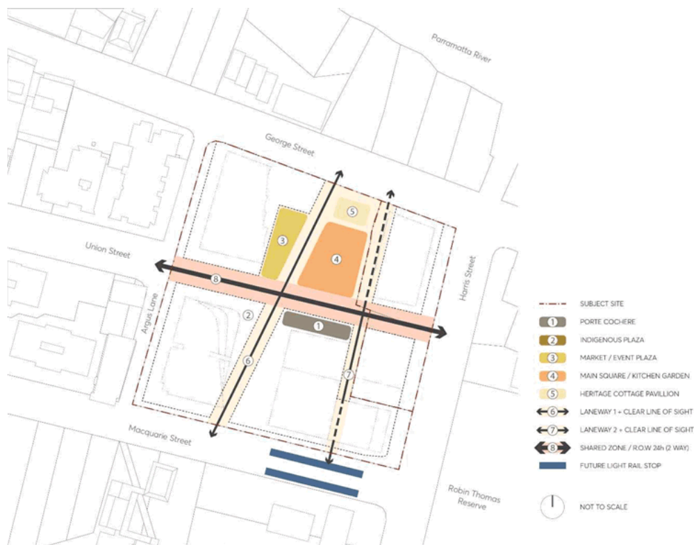
Figure 4.3.3.7.31 – Control diagram: Pedestrian links and shared zones
