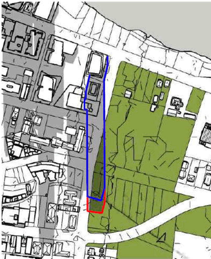
Figure 11: overshadowing caused by the Albion Hotel site at 12pm on 21 June. (Blue line reflects shadow profile of 149.5m tower. Red line reflects shadow profile of 166m tower).
