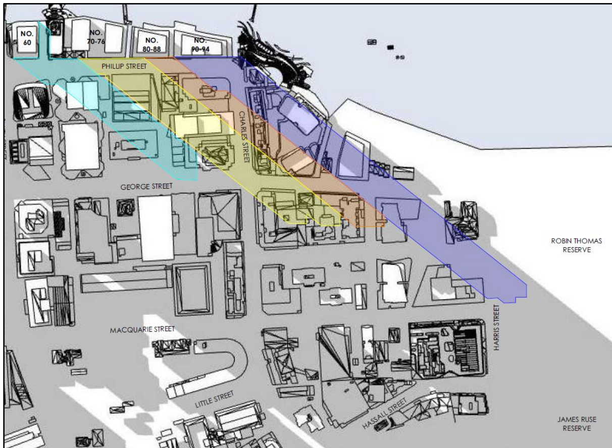
Figure 11: Extract from shadow diagrams showing shadows cast at 3.00pm on 21 June (Source: Applicant's Reference Scheme – PTI Architecture). Shadow from subject site is shown in dark blue. Shadows from currently permissible development shown in grey shading.
