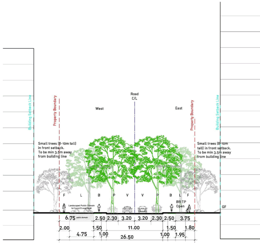
Figure 8.2.6.3.1.5 – Type 2B Main Road with Cycle Tracks between EWR 4 and EWR 6 (NSR 3)
