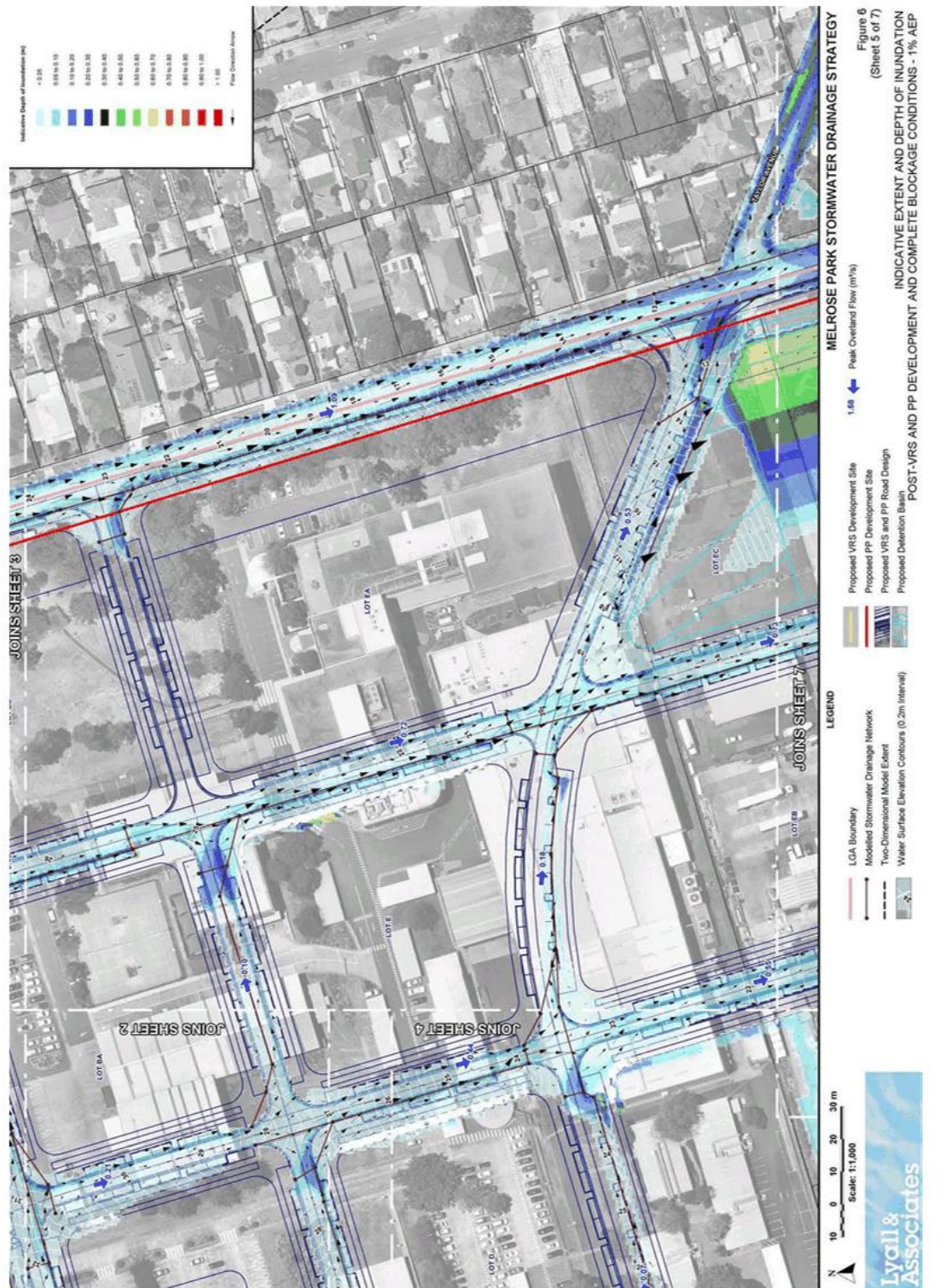
Figure 8.2.6.8.4 – Melrose Park Stormwater Sheet 4 (Source: Lyall & Associates)
