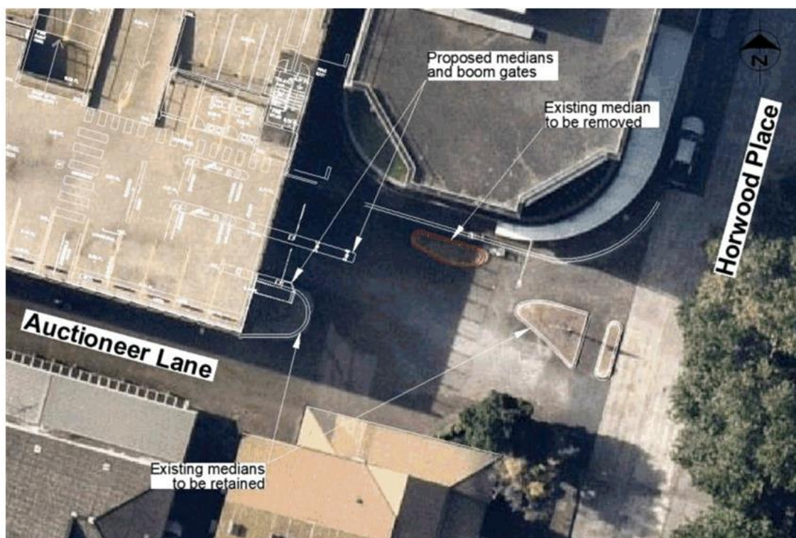
Figure 2: Proposed construction of concrete medians and boom gates within Auctioneer Lane
