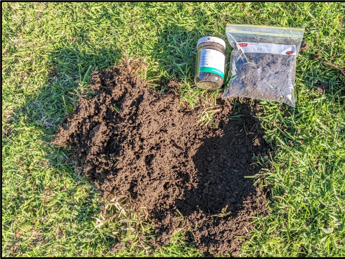
Figure 17. TP3 test pit excavation and sampling.
