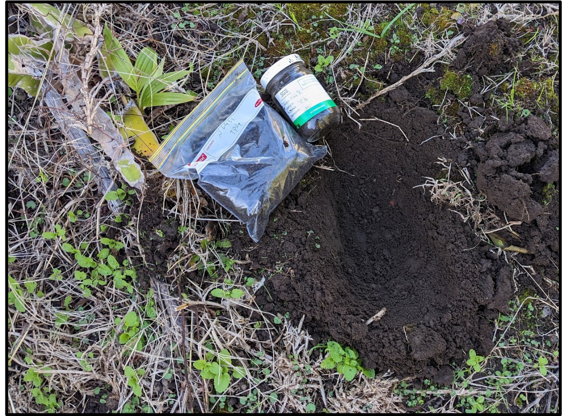
Figure 18. TP4 test pit excavation and sampling.
