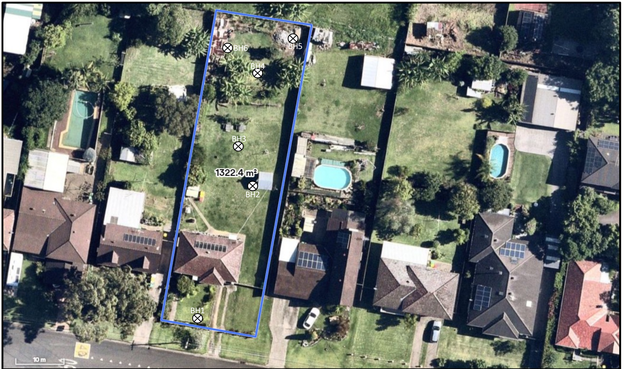
Figure 2. The approximate area of the site is 1,322m 2 . Six (6) soil samples were obtained from six (6) test pits across the site.
