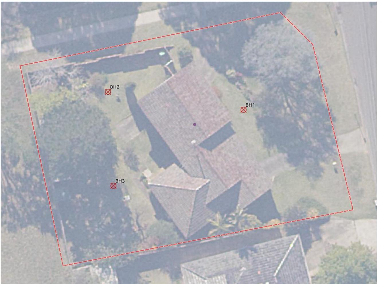
**Figure 2-6:** Aerial image denoting site boundary and bore hole locations
