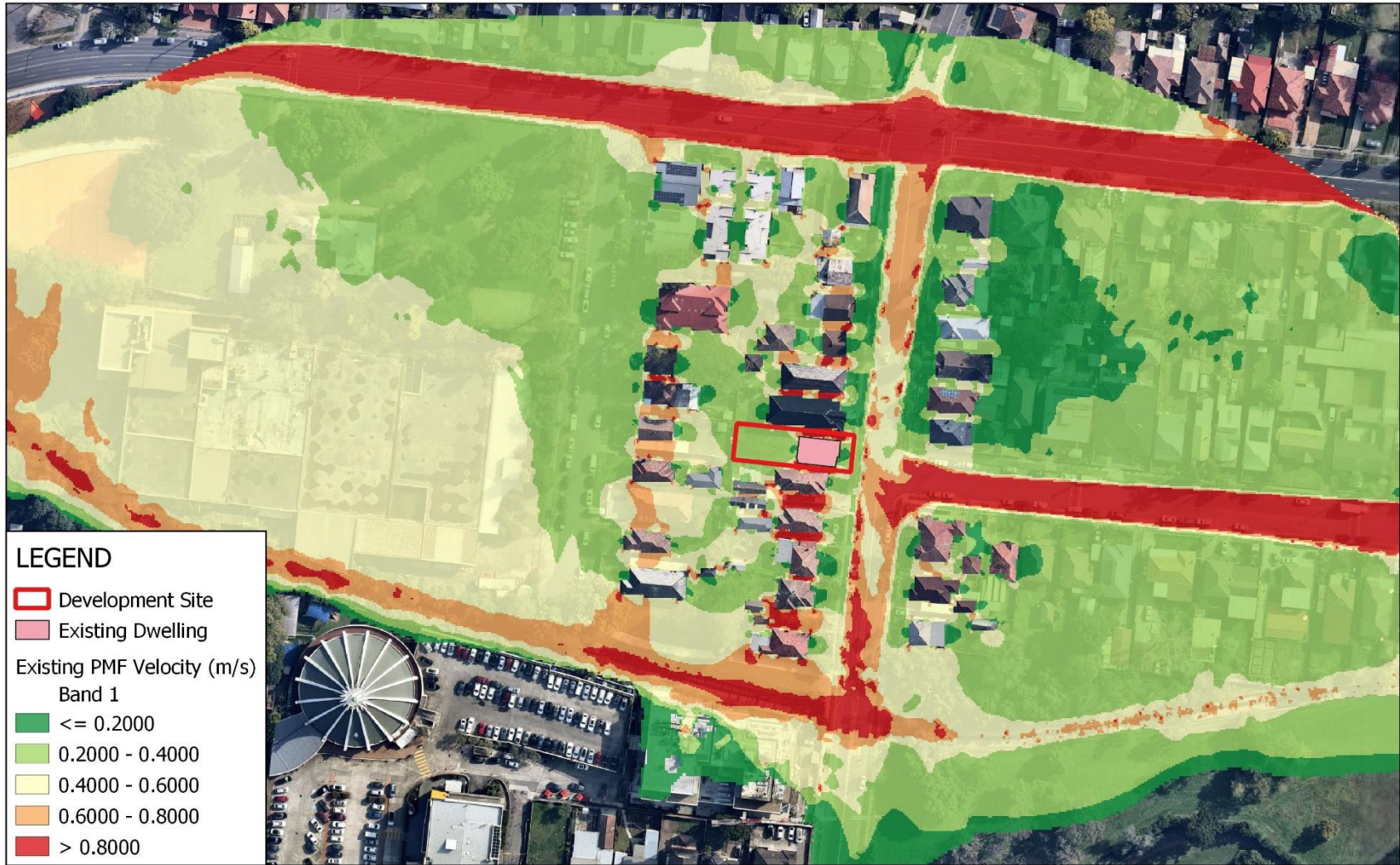
Figure 19: Existing Condition PMF Velocity Map
