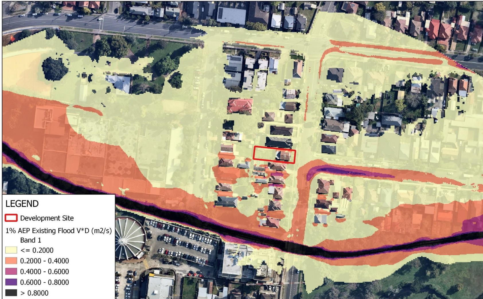
Figure 16: 1% AEP Existing Condition Velocity Depth Product ( V \cdot D ) Map
