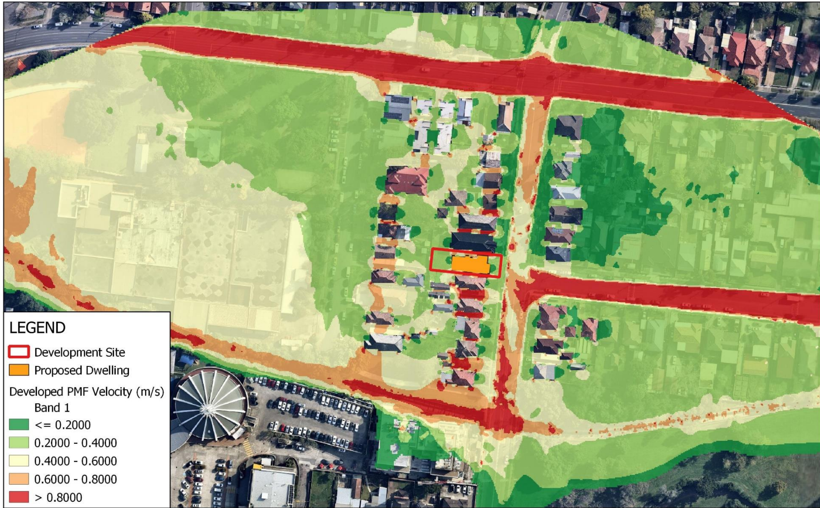
Figure 28: 1% AEP Developed Condition PMF Velocity Map
