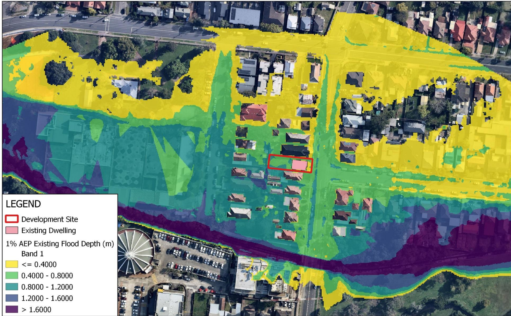
Figure 14: 1% AEP Existing Condition Flood Depth Map
