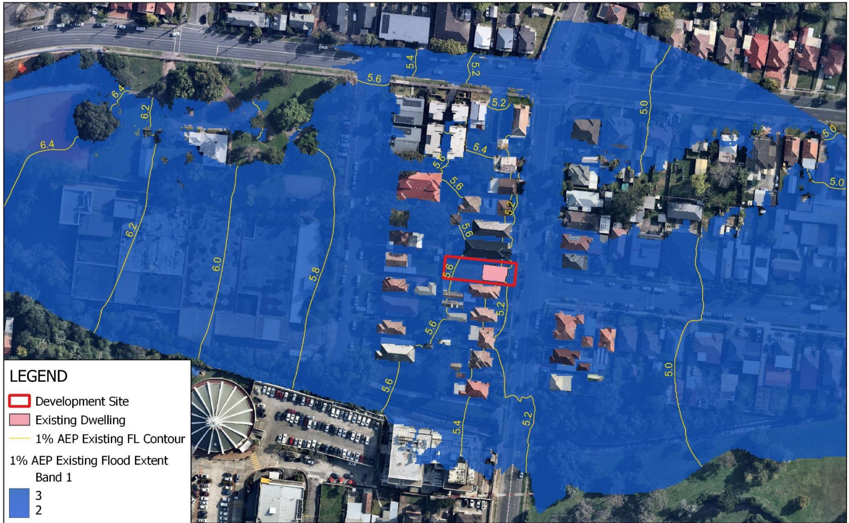
Figure 13: 1% AEP Existing Condition Flood Extent with Flood Level Contour
