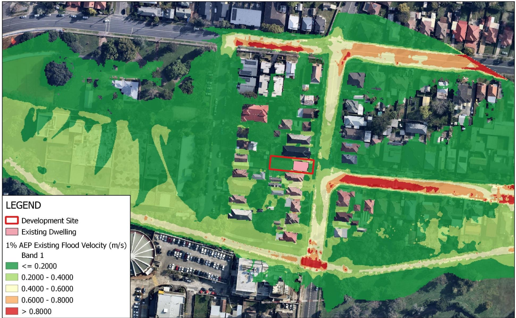
Figure 15: 1% AEP Existing Condition Flood Velocity Map
