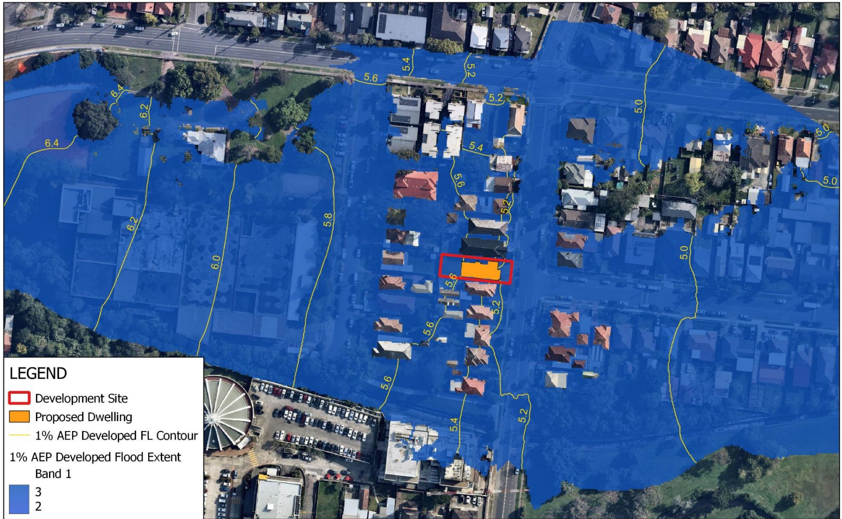
Figure 22: 1% AEP Developed Condition Flood Extent with Flood Level Contours
