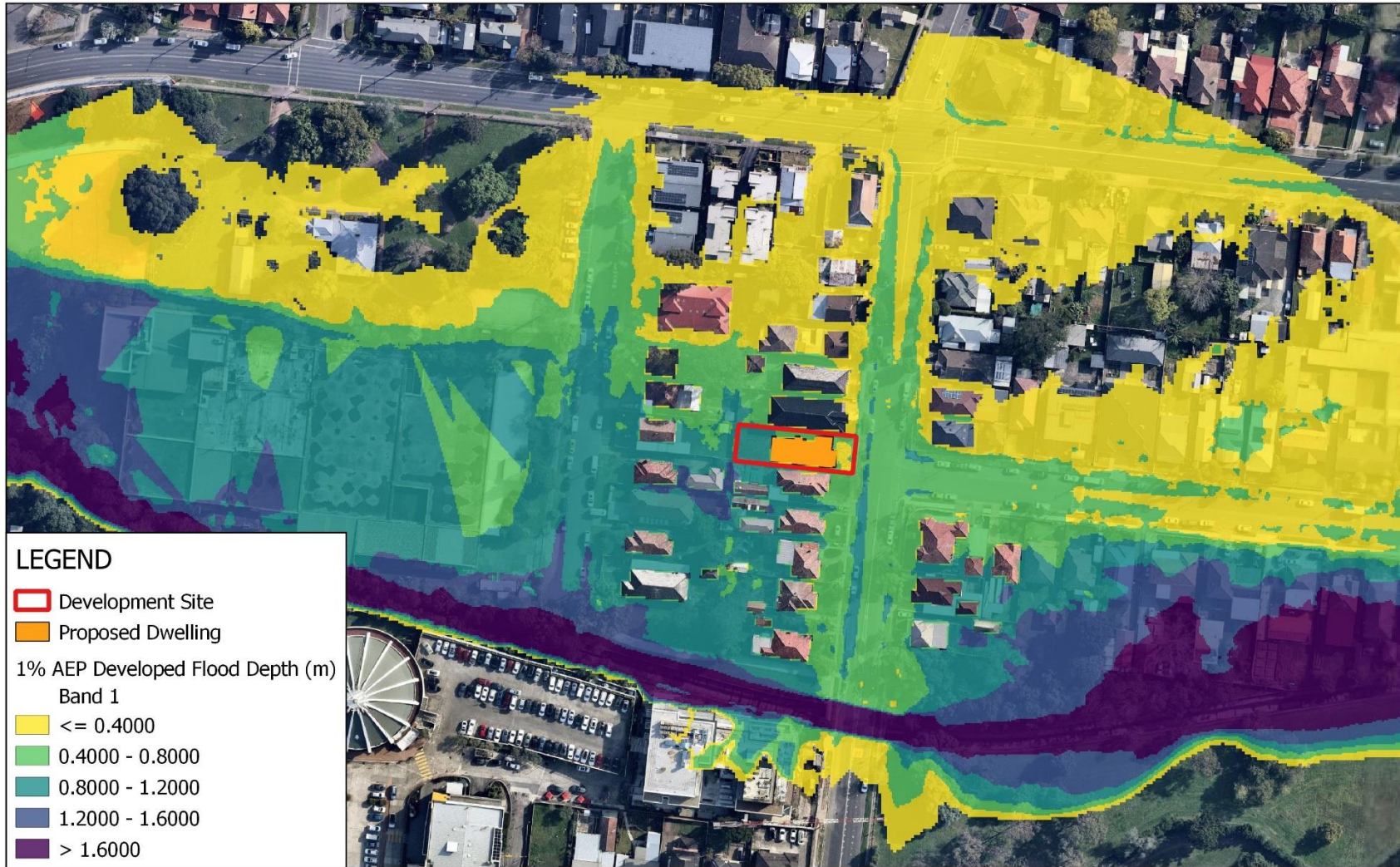
Figure 23: 1% AEP Developed Condition Flood Depth Map
