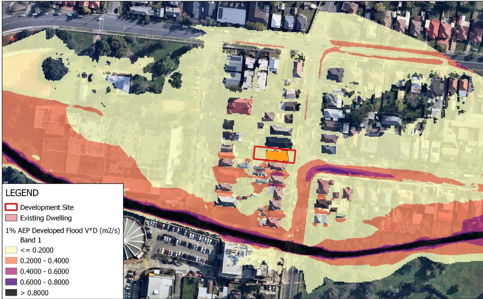
Figure 25: 1% AEP Developed Condition Flood Hazard (Velocity Depth Product) Map
