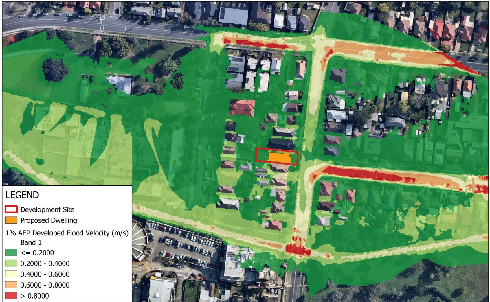
Figure 24: 1% AEP Developed Condition Flood Velocity Map
