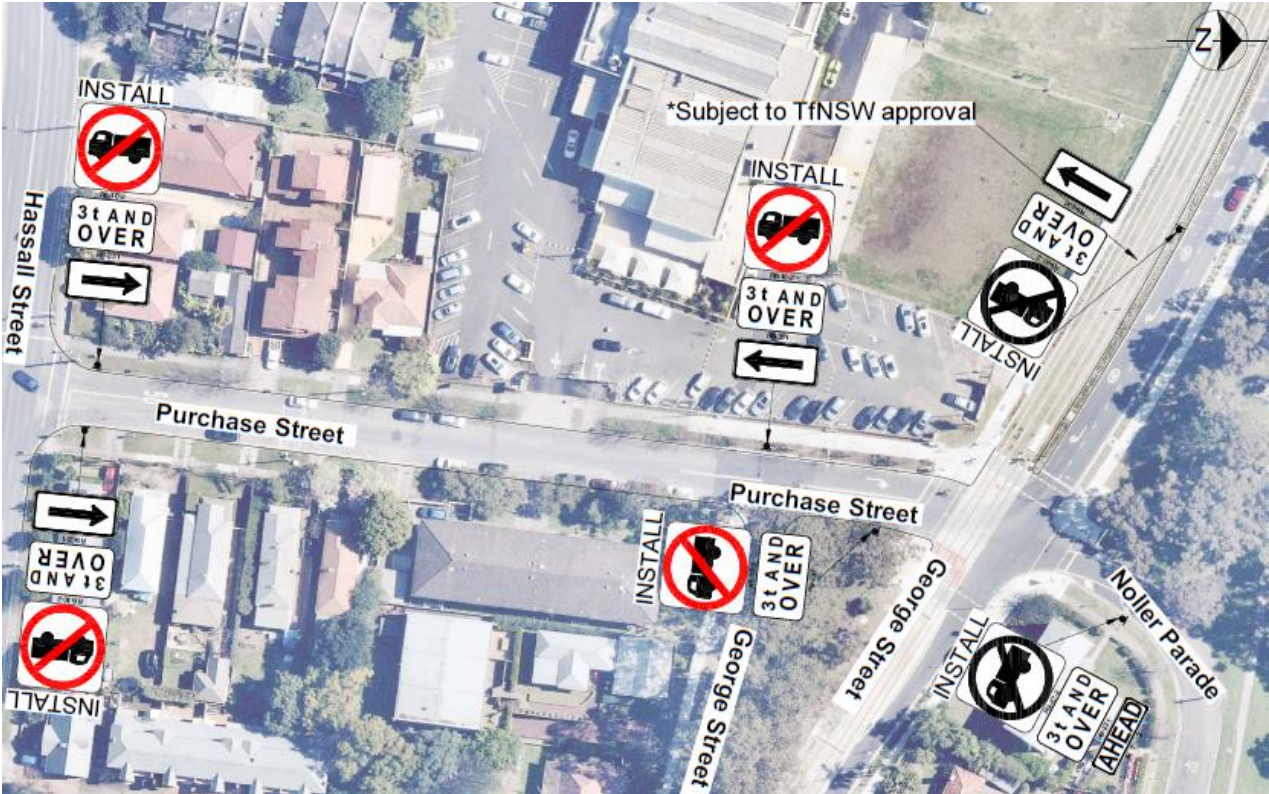
Figure 2: Concept plan of the proposed 'No Trucks - 3t and Over' load limit restriction in Purchase Street, Parramatta
