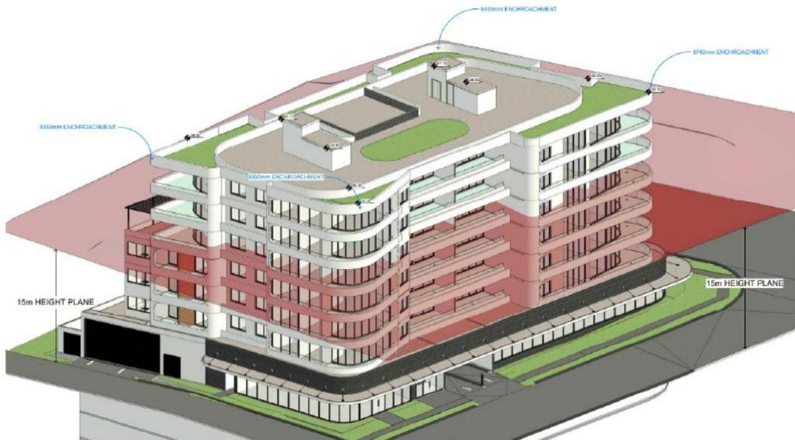
**Figure 15. Height plane diagram**
