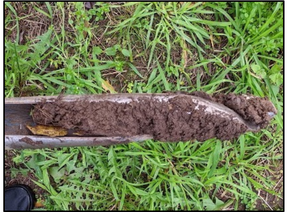
Figure 14. BH3 sample profile consisted of dark brown medium clay within the fill layer.
