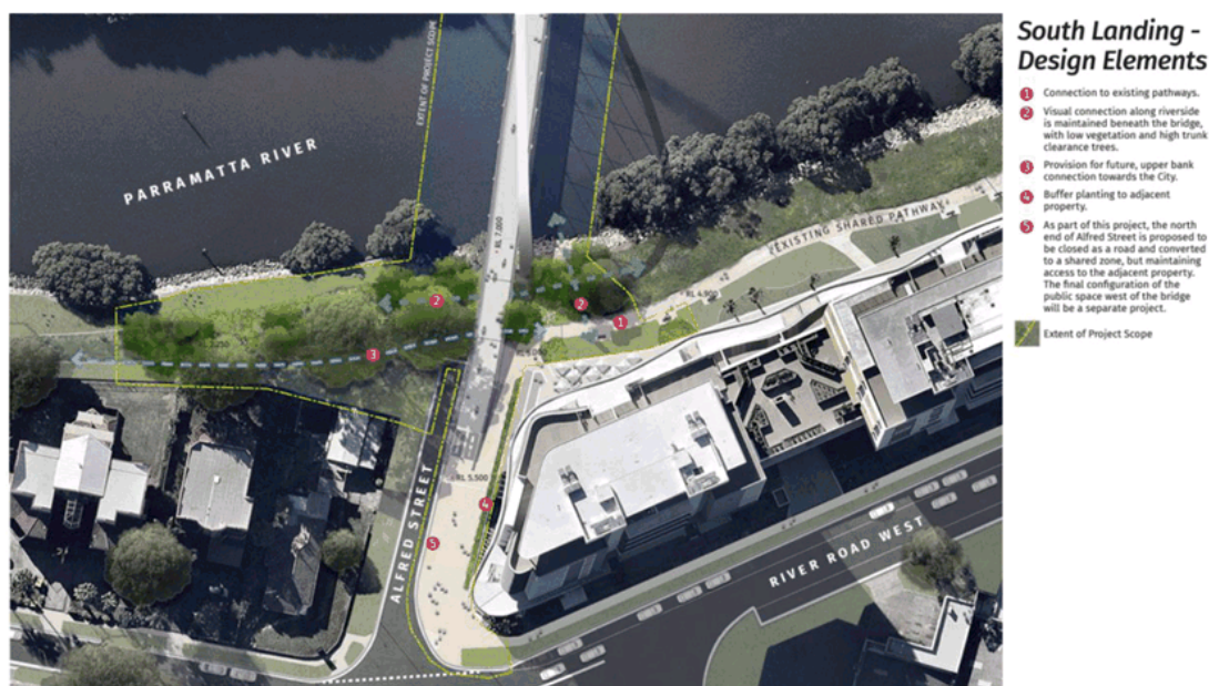
Figure 6 – Artist impression of south landing of the Alfred Street Bridge design elements, which would be supported by funding received as a result of the draft Planning Agreement.
